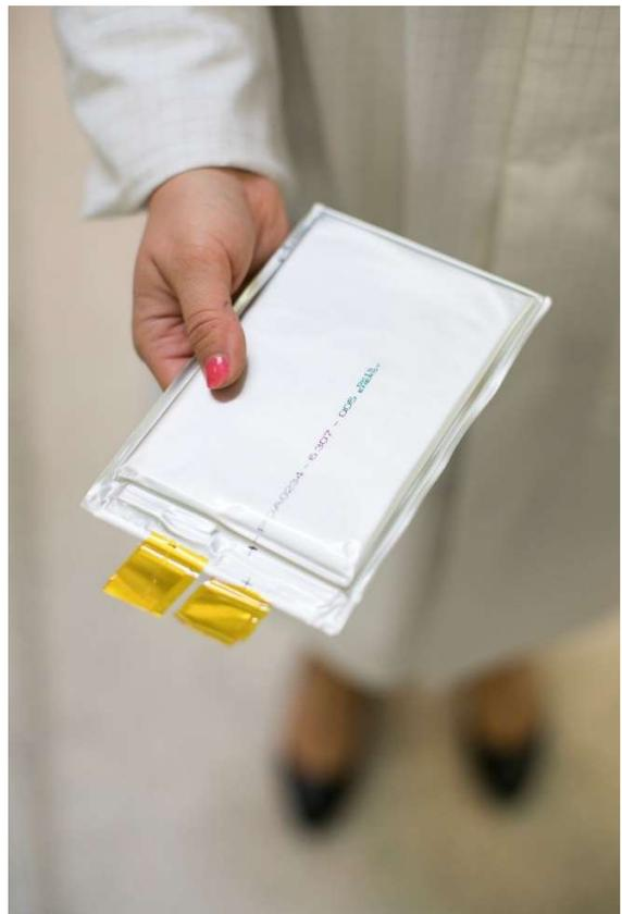
The first generation Quasi Solid-State Li-S cell at 450Wh/kg Specific energy with an Energy density of 550 Wh/L will be delivered by the Summer of 2022. A target of 550Wh/kg, 700Wh/L has already been set for the Autumn of 2023. The above key performance indicators have been agreed commercially between OXIS and Sanyo Trading company Ltd of Japan to meet customer requirements for the Japanese market. The cell capacity will range between 10-20 Ah.
